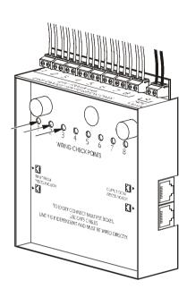
c. As a final test, apply power to all InfraStruXure and auxiliary devices, and then press the EPO button. All connected devices should power OFF immediately. Repeat this final test at every EPO box in your system.
