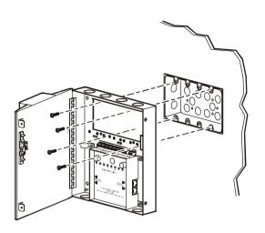
7. Reinforce the EPO box with \(^1\sqrt{4}\)-inch screws in the corner mounting holes. (See page 14 for a schematic of the EPO box mounting holes.)
