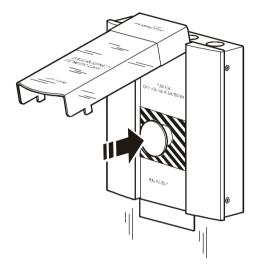
**To reset the EPO system**: Pull the button toward you. Pulling the button does not bring power back to connected equipment; it only resets the EPO system.
