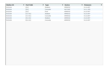
The Browser UI's System page provides detailed information about the devices (KVM switches, Console Modules, and KVM Adapter Cables) deployed on the matrix KVM switch installation.
