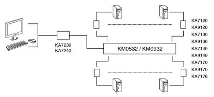
A separate console module is required for each KVM console; likewise, a separate KVM adapter cable is required for each computer. For a listing of compatible console modules, see *Consoles*, page 4. For a listing of compatible KVM adapter cables, see *Cables*, page 5.
