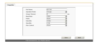
4. Drop down each of the serial parameter lists to select the port property values that match the ones used by the connected serial console device. The port property settings that the KA7140 supports are given in the following table:
