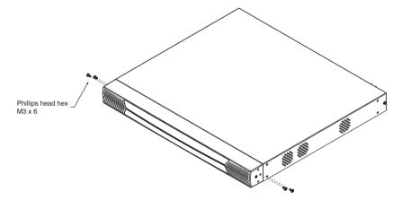
2. Use the M3 x 8 Phillips head hex screws supplied with the rack mount kit to screw the rack mounting brackets into the front of the unit:
