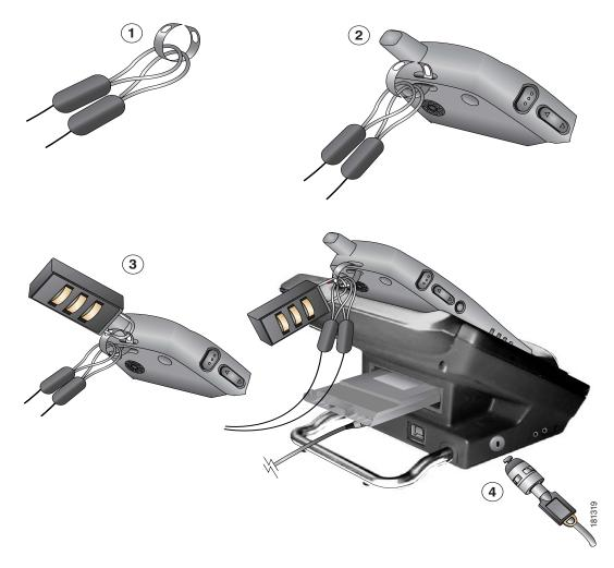
You can secure your Cisco Unified Wireless IP Phone 7921G Desktop Charger by using a laptop cable lock. The lock connects to the security slot on the side of the desktop charger, and the cable can be secured to a desktop. The diagram shows where to insert the lock.
