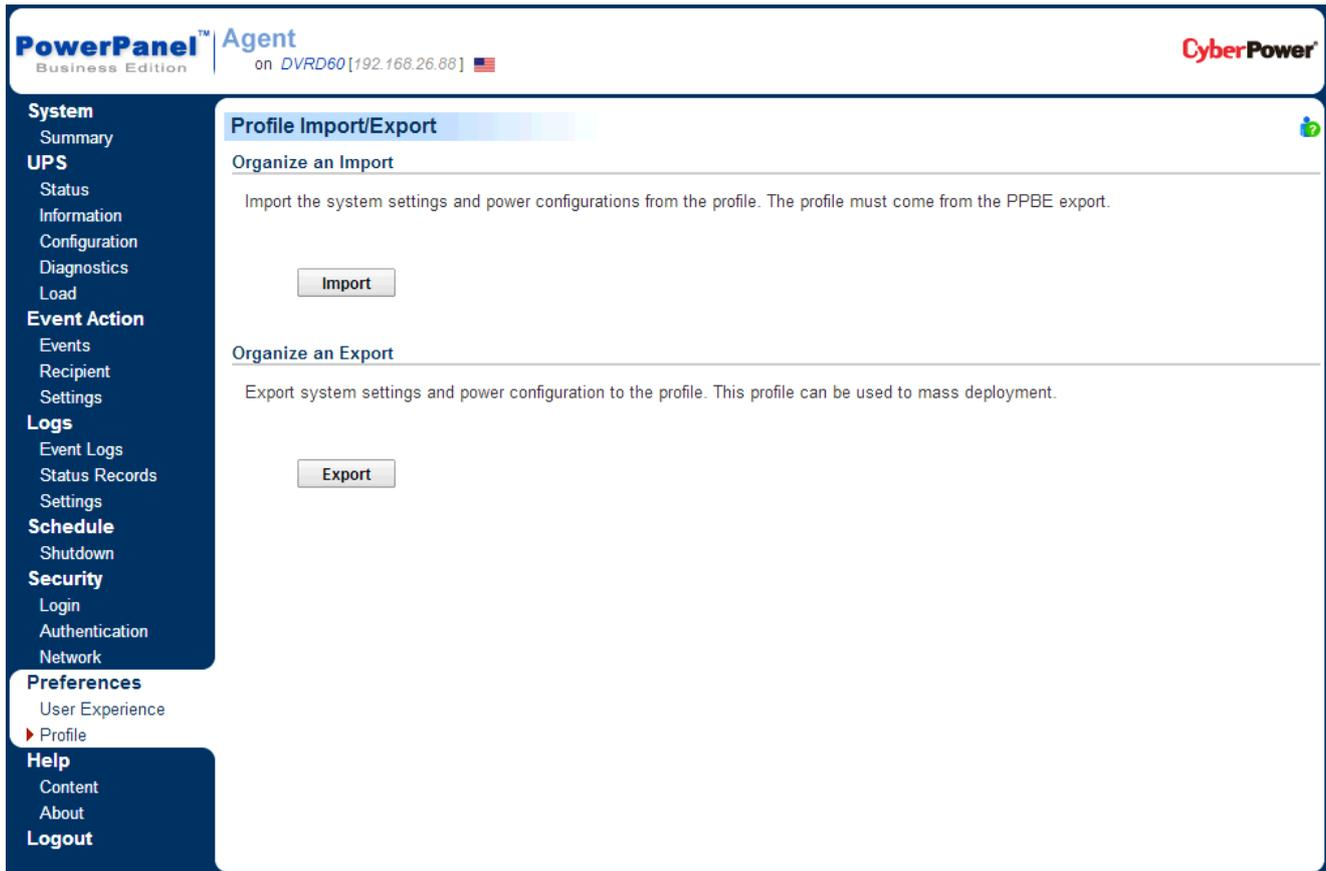
In order for administrators to do mass deployment, **Profile** page allows to export all power configuration and system settings from the target computer. Each computer running PowerPanel Business Edition can import this profile to apply the same power configuration and system settings.
