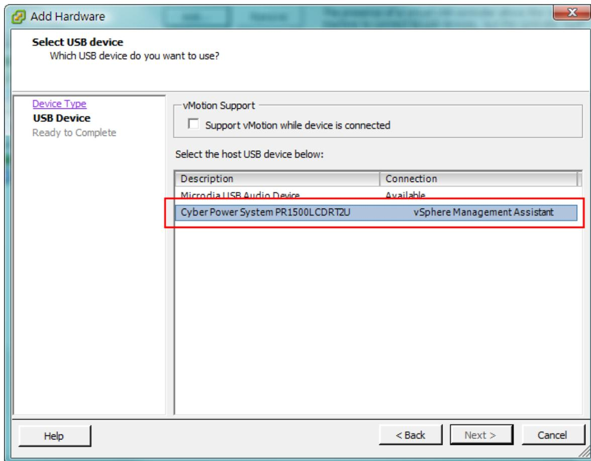
**Note:** In order to make sure that USB device of the target UPS can connect to vMA after a USB controller is added, it is strongly recommended to upgrade the virtual hardware to the latest version prior to adding a USB controller and a USB device. See [How do I upgrade the virtual hardware version of vMA](#) for details.
