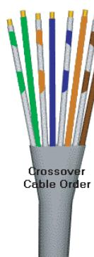
**Then when the pairs are inserted into the RJ45 plug they should look like this:**
