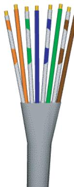
**Then when the pairs are inserted into the RJ45 plug they should look like this:**
