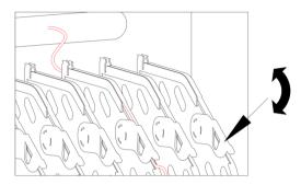
10. Place tablets or laptop one by one in the tablet (laptop) slot and connect to the corresponding data cable
