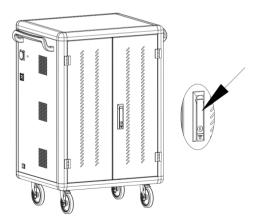
Plug your tablet or laptop charger into the socket at the back of the car one by one, then thread the cable through the hole. For laptop charges, place the adapter in the bucket below the thread hole
