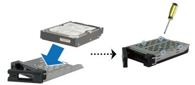
• For 2.5" drives: Place the drive in the drive tray. Turn the tray upside down and tighten screws into the four spots indicated below to secure the drive in place.
