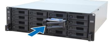
Note: Make sure that the drive tray is completely inserted. Otherwise, the drive might not function properly.
