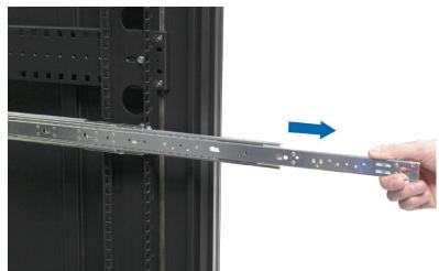
3 Align the fixing holes of the inner rail to the side of the chassis and slide backward to attach the inner rail.
