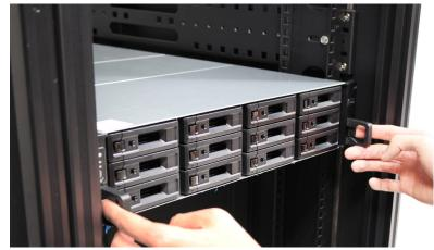
2 With the help of another person, carefully remove the chassis from the rack. Then, slide forward to remove the inner rail from the chassis.
