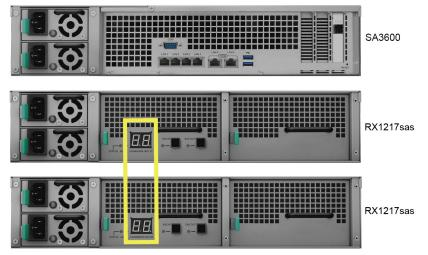
**Note:** Even with the Synology NAS and expansion unit(s) powered on, you can still expand with one or more expansion unit if needed. To do so, repeat above steps to connect the expansion cables and power cords of the other expansion units. Your expansion units will automatically power on if they are correctly connected, and the expansion unit ID will be displayed accordingly after a few seconds (if DSM is correctly installed in the Synology NAS server).
