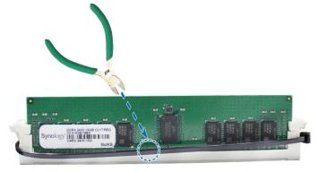
Note: Avoid touching any components of the motherboard when you cut the cable tie.
