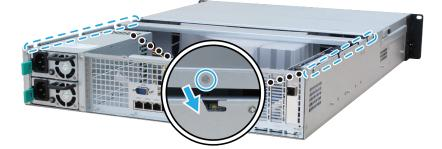
**b** Put back and fasten the screw you removed in step 2.
