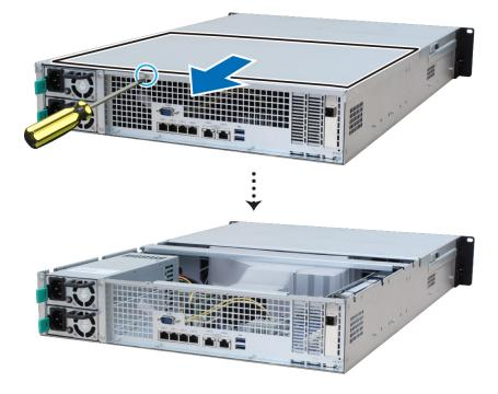
**Note:** When you remove the rear top cover, sensitive internal components are exposed. Avoid touching anything other than the memory assembly when you remove or add memory.
