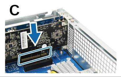
*Note:* Make sure the connector is fully inserted. Otherwise, the network interface card might not be able to function properly.
