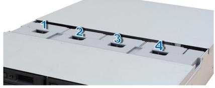
4 Find the malfunctioning fan. Lift the fan upward to remove it.
